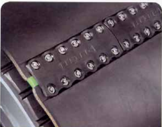
Figure 5. Rubber covered fasteners, such as Flexco® VP fasteners are ideal for use with belt cleaners and highly abrasive materials.
