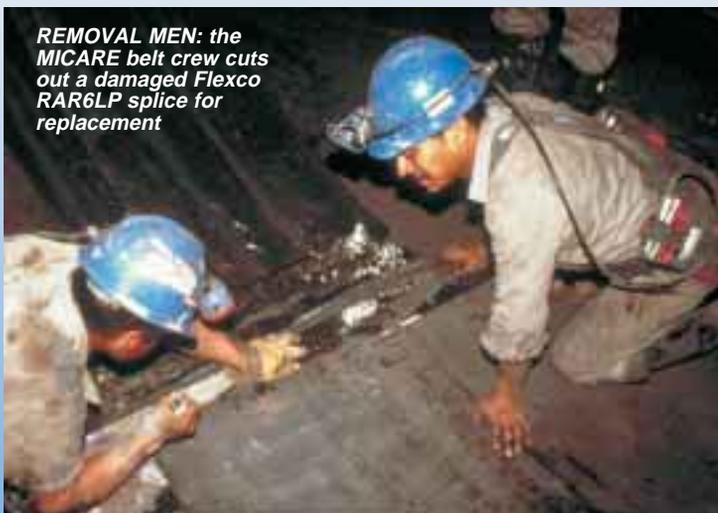
**REMOVAL MEN:** the MICARE belt crew cuts out a damaged Flexco RAR6LP splice for replacement
