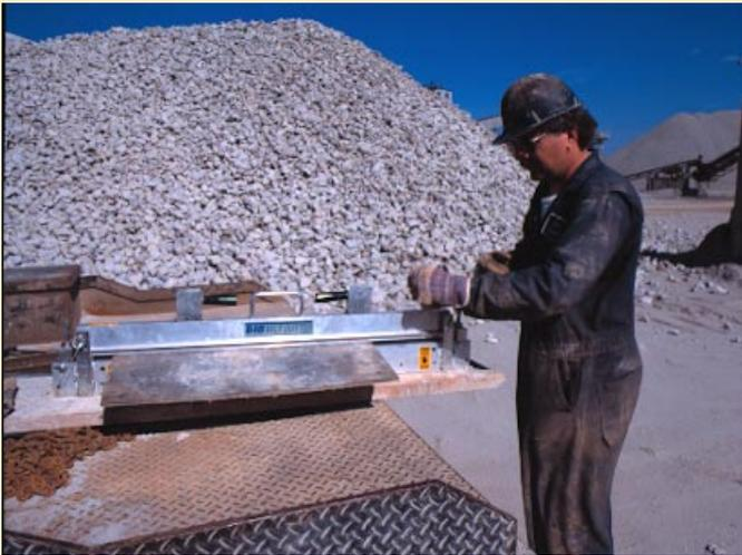
Shown in action at Nelson Aggregate's Burlington Quarry, the Flexco 840 series belt cutter safely delivers a controlled straight cut.
