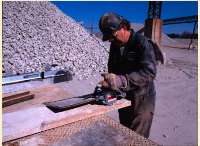
Flexco's FSK belt skiver is designed to extend the life of mechanical joints and reduce component wear.
