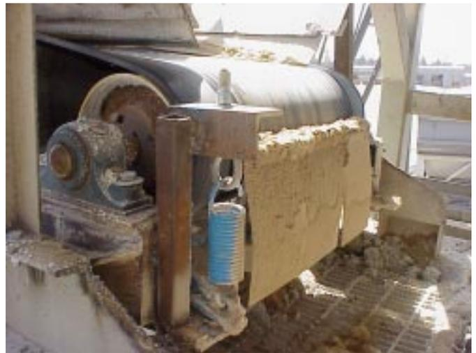
In rest position outside the kiln, slinger head-end shows why stainless steel blade-tip shields are needed to keep buildup off cleaner-blade mounting bolts for easier blade replacement.
