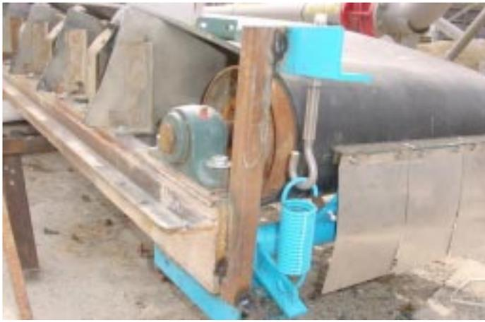
Installation of Flexco Eliminator® H-Type® high temperature belt cleaner at the head pulley of a moveable slinger shows tungsten-steel blades mounted higher than usual, with cross-pole blade mount and spring tensioning mechanism trimmed to fit within slinger's moving inner carriage.
