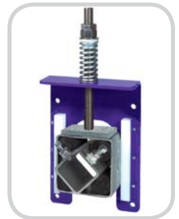
A self-contained spring tensioner delivers constant tensioning power to the cushions and blades for consistent blade-to-belt contact.
